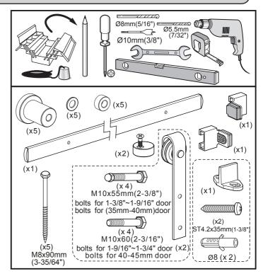
To obtain the maximum weight capacity, all rail mounting fasteners must be mounted directly into solid wood. Do NOT install directly onto a drywall surface. A solid wood header is recommended as shown in instruction box 2.
